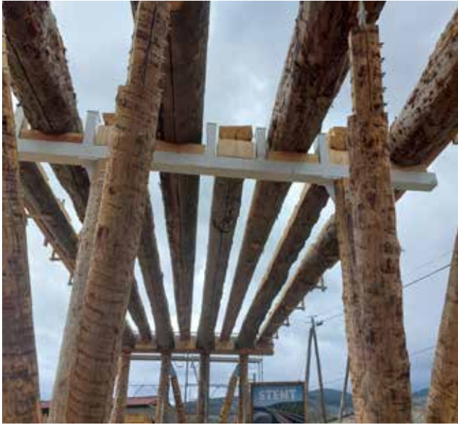
Large prototype 6x16m for bending and vibration testing.
